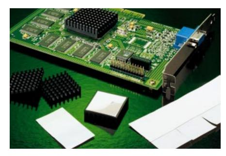
providing a high adhesive strength attachment for heat sinks. The high performance silicone PSA allows adhesion to silicone-contaminated plastics and other low energy surfaces.
