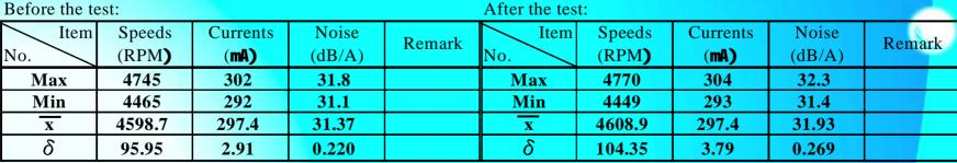
Result: After the performance test, 30pcs fans of speeds, currents and noise all meets the specifications, test is ok.
